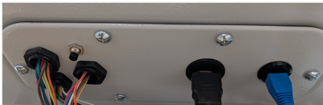
FIG. 5 · BOTTOM PANEL – RESET BUTTON (CENTER), HDMI (PRO), AND ETHERNET (CONNECTED & PRO).
